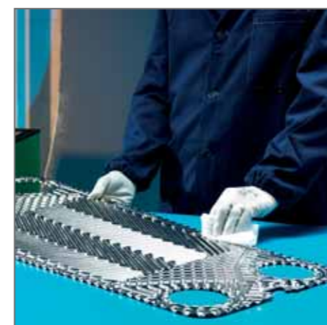
4. Cleaning gasket seal seats
