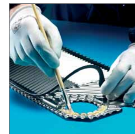
10. Gasket gluing procedure
