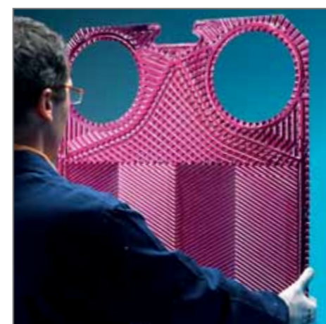
5. Micro hole detection with penetrating liquids
