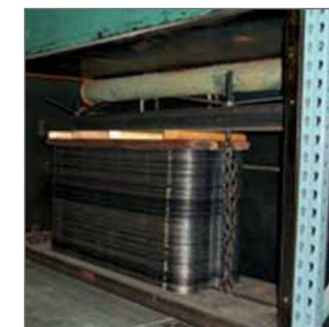
11. Plate pack pressing with adhesive glue polymerisation in the oven
